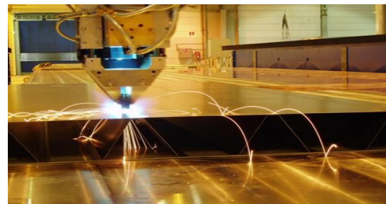
Laser3 - welding of metallic lightweight sandwich panels
