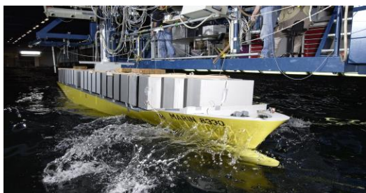
Model tests of Emma Maersk , one of the largest containerships
